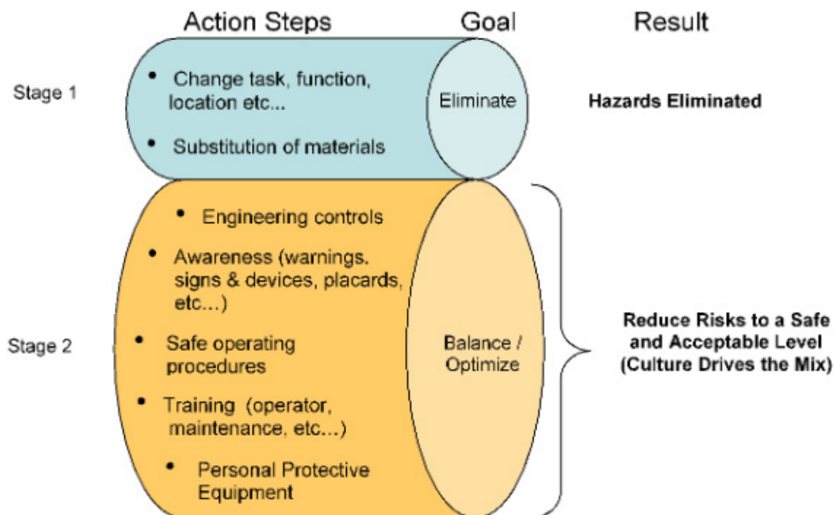
Figure 3. Two-Stage Iterative Approach to the Hierarchy of Controls and Risk Reduction
