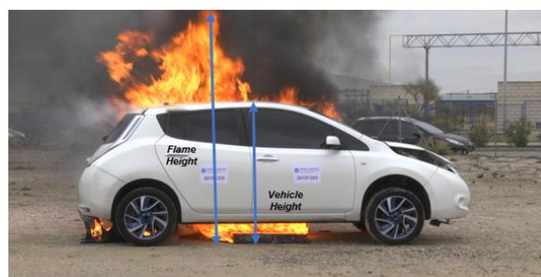
**Figure 20.** Image of an instant of the fire test in which the height of the flame is measured (time elapsed 7.33 min).
