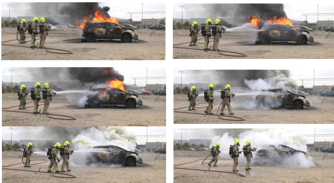
**Figure 28.** Images of the Nissan Leaf vehicle fire smothered with pressurized water and Renault's Fireman Access idea.
