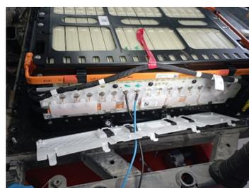
Wiring placement on the + and – poles to perform overload with an external power supply.
