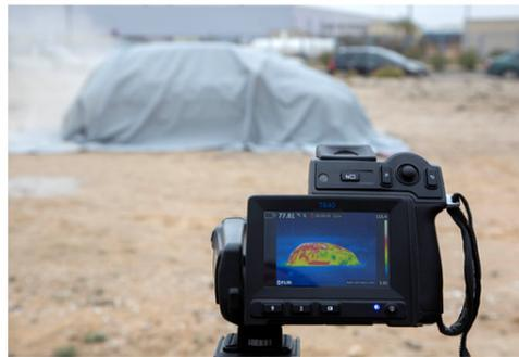
**Figure 11.** Thermal imaging camera image to record and document the vehicle's temperature during the test.
