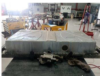
High-voltage battery of the Smart EQ ForFour vehicle removed for instrumentation.
