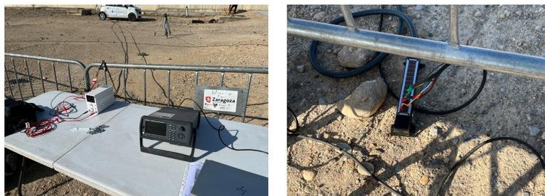
**Figure 8.** Location of the portable detectors around the vehicle (gas detection), the external charging source, and the Keysight 970 A Datalogger temperature measuring equipment, relative to the vehicle being tested (left). Details of the thermocouple connection panel (right).
