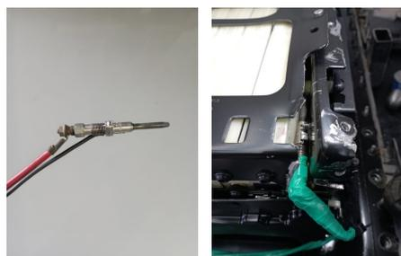
**Figure 6.** Image of the diesel engine heater used (left) and detail of the area where the heater was placed on the battery (right).
