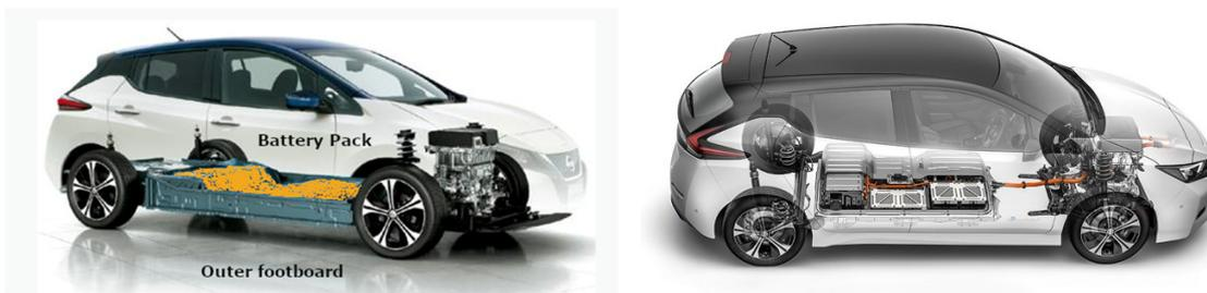
**Figure 1.** Electric vehicle used during the tests (left) and location of the high-voltage battery (right).
