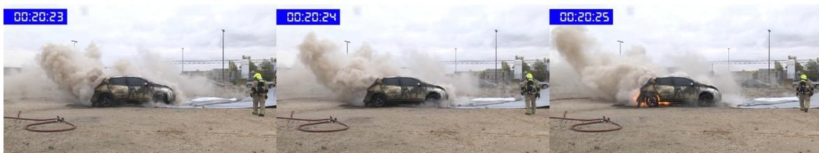
**Figure 12.** Frames of the moment when the fire restarts after the vehicle is discovered.
