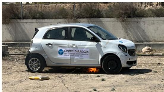
**Figure 7.** Location of the fossil fuel burner placed on the underside of the Smart EQ ForFour vehicle to start the fire.
