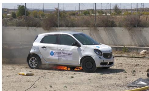
**Figure 29.** Instant of the Smart EQ ForFour vehicle fire test 1 min after the start of the fire.
