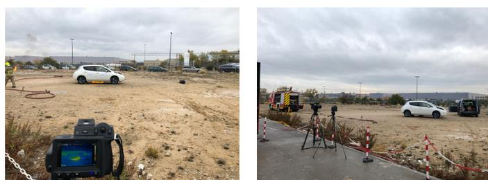
**Figure 2.** Location of the thermal imaging camera and video camera in relation to the tested vehicle.
