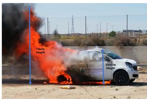
**Figure 39.** Image of an instant of the fire test of the Smart EQ ForFour vehicle in which the height of the flame is at its maximum (2.5 m) (time elapsed 6.01 min).
