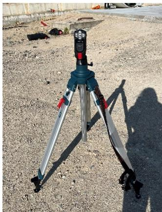
**Figure 41.** Detailed image of a standard portable G7 multi-gas detector from Blackline Safety, used to measure the gases emitted during the fire test.
