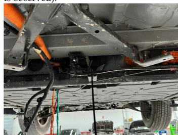
Detail of the wiring placed in the battery to perform the different measurements.
