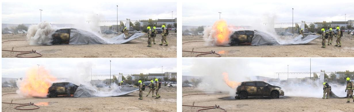
**Figure 25.** Smoke evolution after removing the fire blanket and reactivation of the Nissan Leaf electric vehicle fire.
