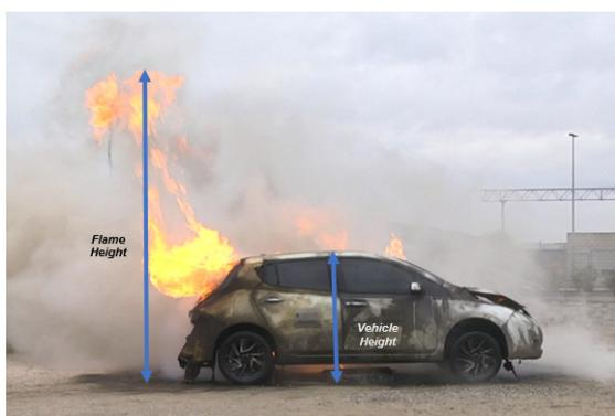
**Figure 22.** Image of the moment when the fire blanket is removed, and the flame reaches a greater height (3.6 m) (time elapsed 21 min).
