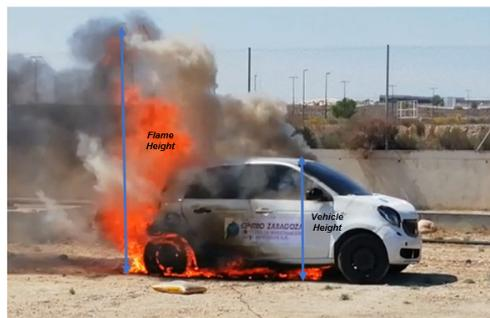
**Figure 38.** Image of an instant of the fire test of the Smart EQ ForFour vehicle in which the height of the flame is measured (time elapsed 3.24 min).
