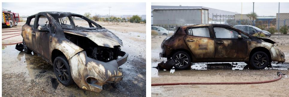
**Figure 15.** Images of the final state of the Nissan Leaf vehicle after the fire test.
