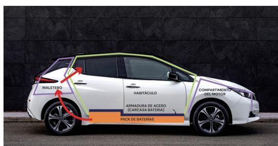
**Figure 17.** Flame and smoke propagation (red arrows) (at the beginning of the Nissan Leaf vehicle fire test).
