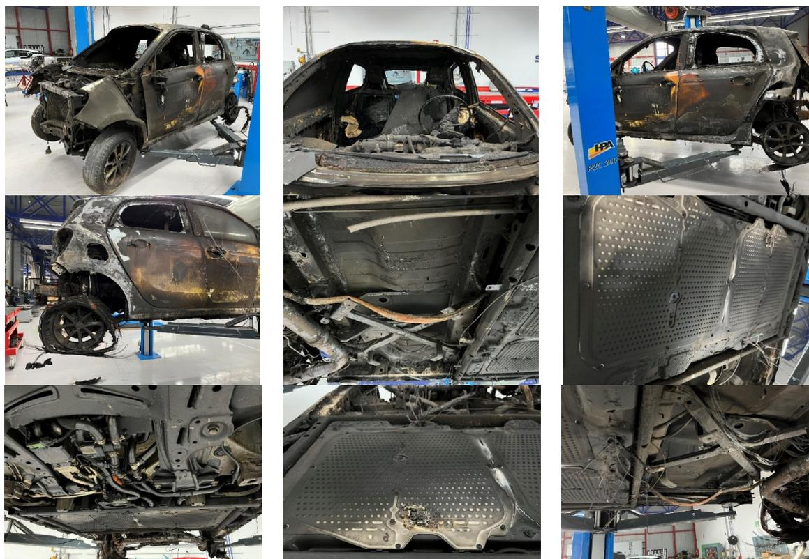
Figure 34. Images of the final state of the Smart EQ ForFour vehicle after the fire test.
