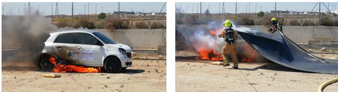
Figure 30. Zaragoza firefighters covering the burning Smart EQ ForFour vehicle with a fire blanket.
