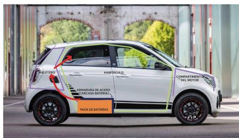
**Figure 35.** Flame and smoke propagation (red arrows) (at the beginning of the fire test) in the case of the Smart EQ For Four vehicle.
