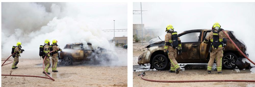
**Figure 14.** Images of the first responders extinguishing the fire with water and cooling the battery to prevent the blaze from re-igniting.
