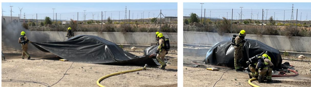
Figure 33. Images of the first responders placing the fire blanket during the vehicle’s fire test.
