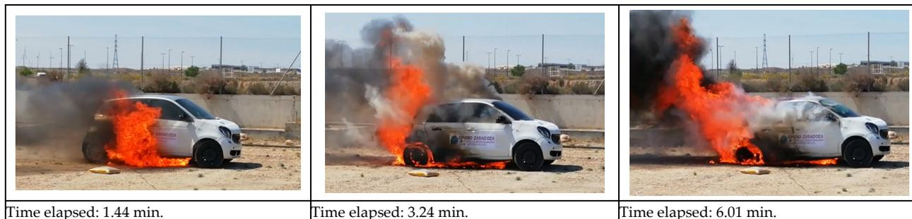
**Figure 36.** Flame height at various times during the fire test (Smart EQ ForFour).
