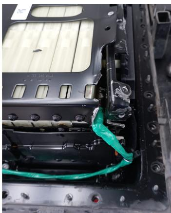
Placing a heater in a cell to cause thermal failure of the cell.
