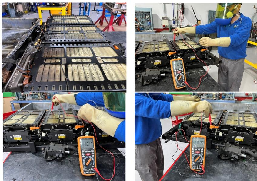
**Figure 46.** Images of the condition of the battery pack, the module, and the lithium-ion cells inside the battery pack.
