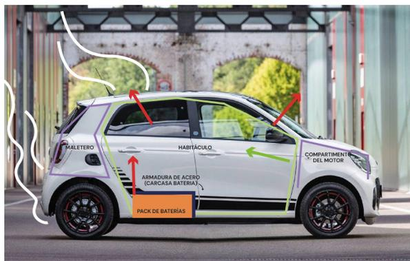
**Figure 37.** Smoke and flame propagation (red arrows and white lines) (at the end of the fire test before putting on the fire blanket) in the case of the Smart EQ ForFour vehicle.
