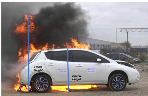
**Figure 21.** Image of an instant of the fire test in which the flame height is at its maximum (2.7 m) (time elapsed 10.06 min).
